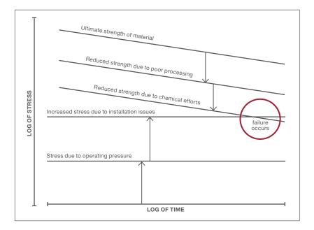
Seldom can one completely predict all the mechanical variables and all the different kinds of chemical substances that will end up inside or on the exterior of a piping system. Therefore, it's prudent for the piping system designer and installer to do what they can to control the various factors that can contribute to environmental stress cracking.
